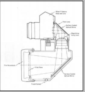
Light travels through the Nikkor lens in use and passes on through the field lens before striking the surface coated optical mirror which sits at a 45 angle to it. From there it through the Eltravels enlarging Nikkor (described as a magnifying relay lens) onto a further optical mirror which in turn reflects it onto the surface of the film within the large format film Quite a journey holder. for light to travel and as one would no doubt expect a loss of light to the tune of 4 stops occurs.
