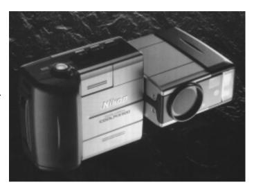
Coolpix 900 with a Nikkor Zoom that covers the equivalent of about 35-115mm. This is a high performance lens with aspheric element to avoid limiting quality. Minimum focus distance is 0.5 metres reducing to just eight centimetres in macro mode (8-50cm),
