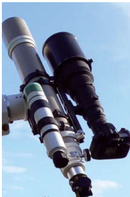
❖ OPPOSITE: Nikkor 500 mm f/4 attached to a 100mm apochromatic f/9 refractor on EQ6 equatorial mount.
