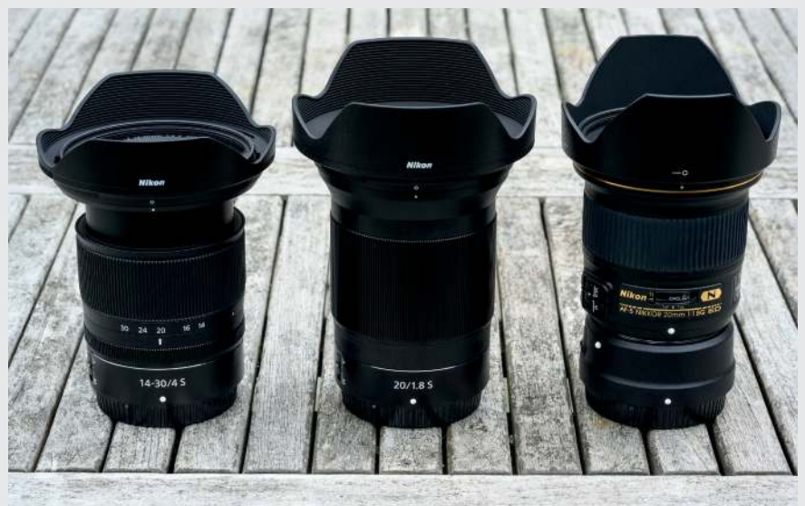
► The Z 20mm f/1.8 S is the largest of the f/1.8 primes released to date, while the AF-S 20mm f/1.8G (right) requires the FTZ adapter; the Z 14-30mm f/4 S lens (left)
