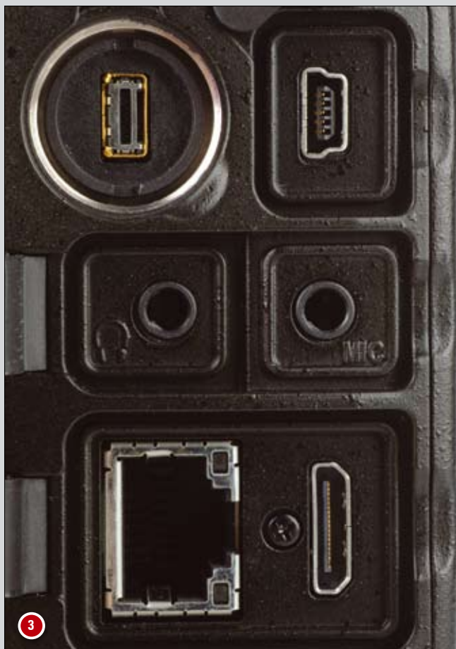
1: The camera has been designed to handle as well when held vertically as it does when held horizontally 2: The D4 is the first D-SLR camera to support the new XQD CompactFlash card specification; its primary card slot accepts XQD cards, while the secondary slot accepts standard CompactFlash cards 3: The D4 offers a plethora of external ports, including a dedicated port for the new WT-5 Wireless Transmitter (top left), for the first time in any D-SLR, an external headphone jack (middle left), and an Ethernet port (bottom left) 4: The WT-5 Wireless Transmitter connects directly to the D4 and draws power from the main camera battery
