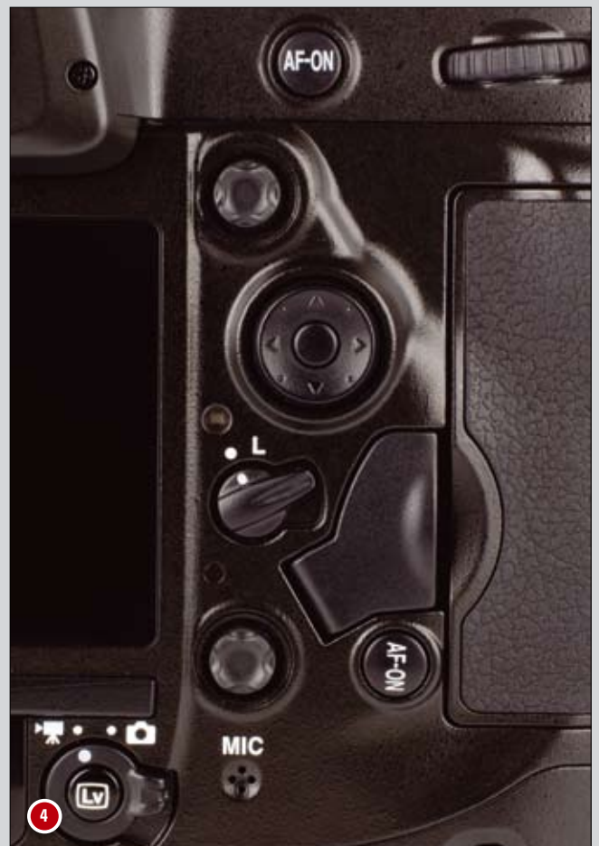
1: The Function and Preview buttons of the D4 can be assigned a range of different roles 2: The angle of the shutter release button is now steeper to help improve camera handling 3: The D4 has adopted the same AF mode and AF-area mode button configuration of the D7000 4: The rear control panel of the D4 is noticeably different from the D3s, with the addition of two buttons for AF point selection
