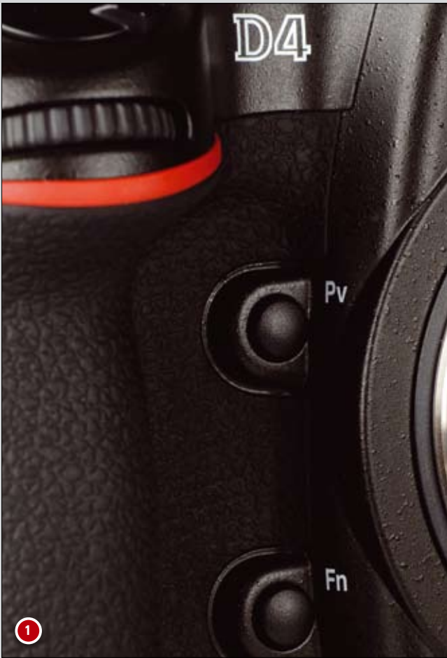
1: The Function and Preview buttons of the D4 can be assigned a range of different roles 2: The angle of the shutter release button is now steeper to help improve camera handling 3: The D4 has adopted the same AF mode and AF-area mode button configuration of the D7000 4: The rear control panel of the D4 is noticeably different from the D3s, with the addition of two buttons for AF point selection
