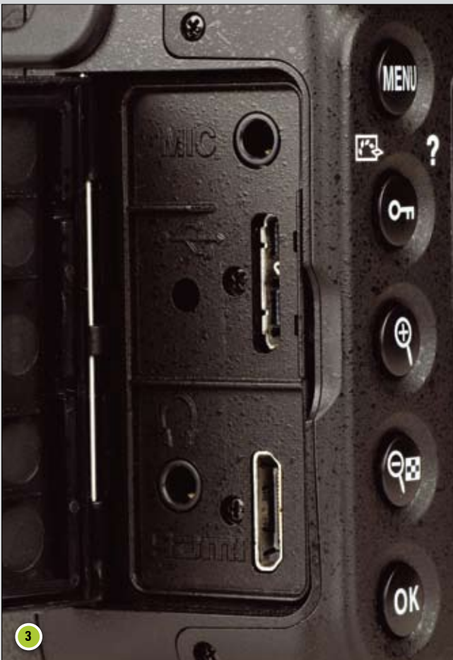
1: External buttons are large and easy to operate 2: The release mode dial now incorporates four buttons 3: The external ports: (from top) external stereo microphone, USB (supports USB 3.0 standard), HDMI and headphone socket 4: The D800 has two memory card ports: one for CompactFlash, the other for Secure Digital
