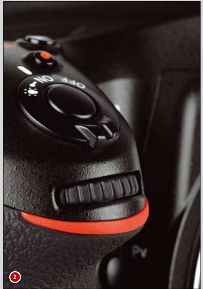
1: The Function and Preview buttons of the D4 can be assigned a range of different roles 2: The angle of the shutter release button is now steeper to help improve camera handling 3: The D4 has adopted the same AF mode and AF-area mode button configuration of the D7000 4: The rear control panel of the D4 is noticeably different from the D3s, with the addition of two buttons for AF point selection
