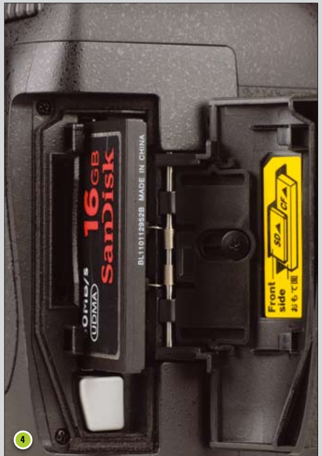
1: External buttons are large and easy to operate 2: The release mode dial now incorporates four buttons 3: The external ports: (from top) external stereo microphone, USB (supports USB 3.0 standard), HDMI and headphone socket 4: The D800 has two memory card ports: one for CompactFlash, the other for Secure Digital
