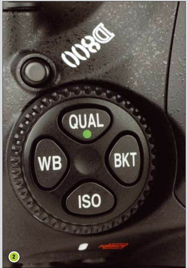
1: External buttons are large and easy to operate 2: The release mode dial now incorporates four buttons 3: The external ports: (from top) external stereo microphone, USB (supports USB 3.0 standard), HDMI and headphone socket 4: The D800 has two memory card ports: one for CompactFlash, the other for Secure Digital
