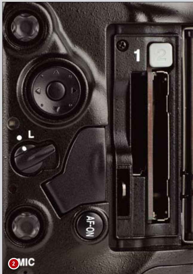
1: The camera has been designed to handle as well when held vertically as it does when held horizontally 2: The D4 is the first D-SLR camera to support the new XQD CompactFlash card specification; its primary card slot accepts XQD cards, while the secondary slot accepts standard CompactFlash cards 3: The D4 offers a plethora of external ports, including a dedicated port for the new WT-5 Wireless Transmitter (top left), for the first time in any D-SLR, an external headphone jack (middle left), and an Ethernet port (bottom left) 4: The WT-5 Wireless Transmitter connects directly to the D4 and draws power from the main camera battery
