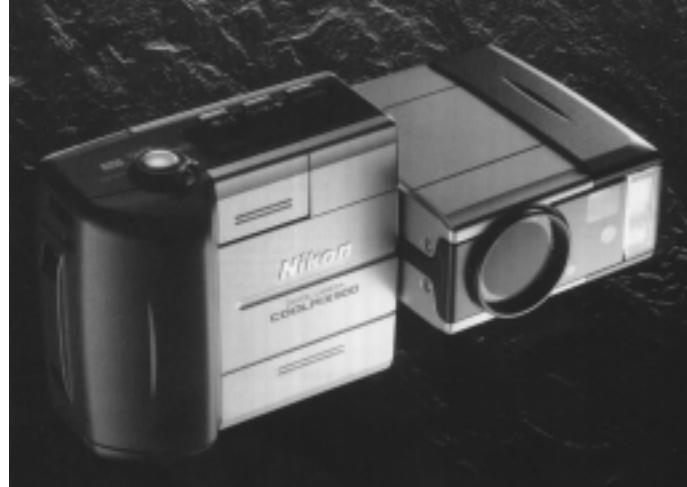
Coolpix 900 with a Nikkor Zoom that covers the equivalent of about 35-115mm. This is a high performance lens with an aspheric element to avoid limiting quality. Minimum focus distance is 0.5 metres reducing to just eight centimetres in macro mode (8-50cm).
