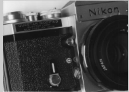
modified for use with the Questar astronomical desk telescope. The photograph of the Questar modified example shows here a narrow black label with white lettering "Questar Modified - Questar Corp. New Hope, PA 18938". This is the only example I have come across with the Questar label. Other examples, such as the Nikon Fs Mr. Rotoloni mentions in his article had no such label.
